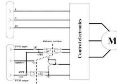
5.4.2 PWM input signal (P1 heating)
